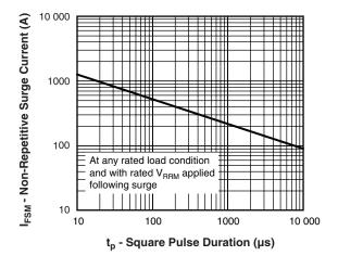
Fig. 7 - Maximum Peak Surge Forward Current vs. Pulse Duration
