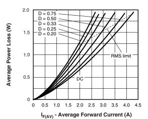
Fig. 6 - Maximum Average Forward Dissipation vs.
