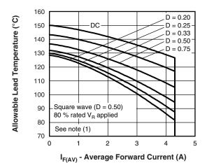
Fig. 5 - Maximum Average Forward Current vs. Allowable Lead Temperature
