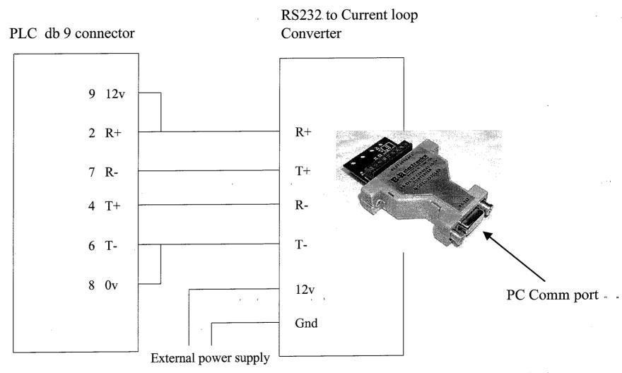
The converter used in this example is manufactured by: B&B Electronics. Their website is www.bb-elec.com.
